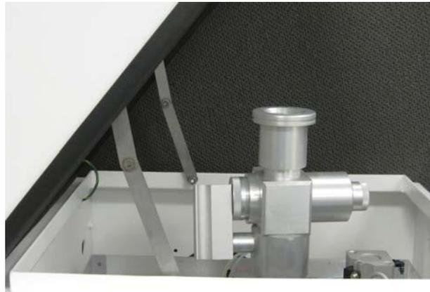
**Figure 10: Removing the Very Sharp Cut Cyclone**
