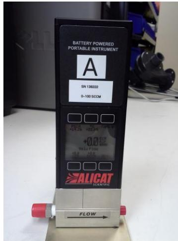
**Figure 3: Alicat MBS Precision Gas Mass Flow Meter**
